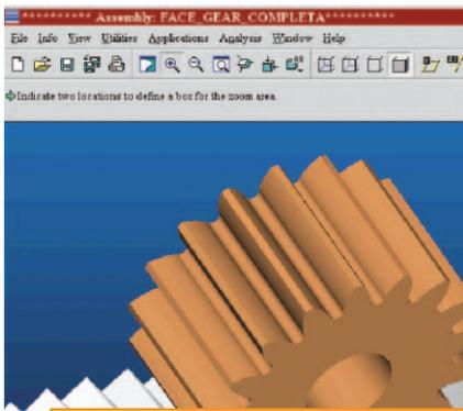
4. Modello CAD 3D del face gear.
